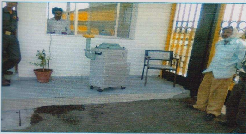
Plate 4: Air Quality Monitoring using Respirable Dust Sampler
